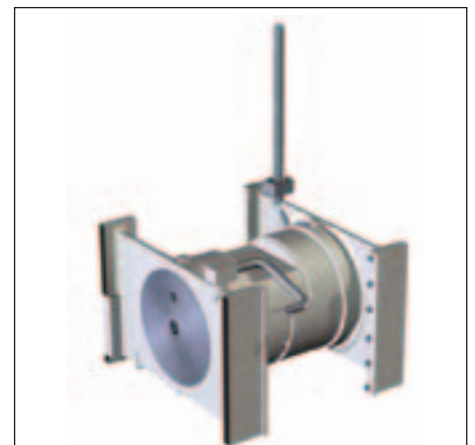
Fig. 16: New crosshead design
